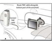
Installation of TMC antenna cable to
